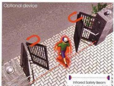
Double safety protection electronic overload sensor and infrared safety beam will stop or reverse the direction if there is an obstacle to the motion.
